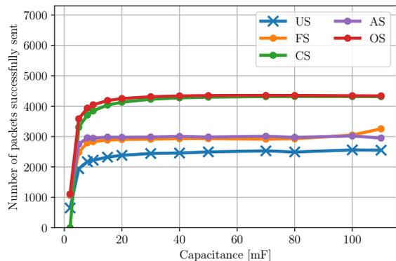
Figure 2: Comparison of scheduling behavior in terms of number of successfully sent packets, for different capacitances and PL=5 B.
